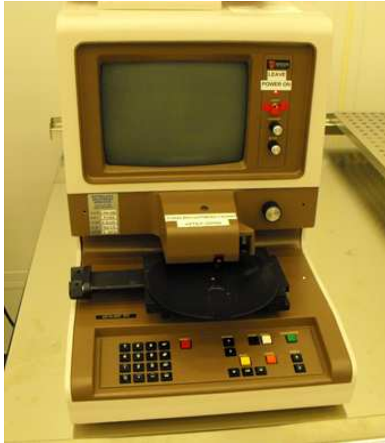
Figure 4.1. Thin film thickness measurement Tencor Alpha-Step 200 profilometer.
